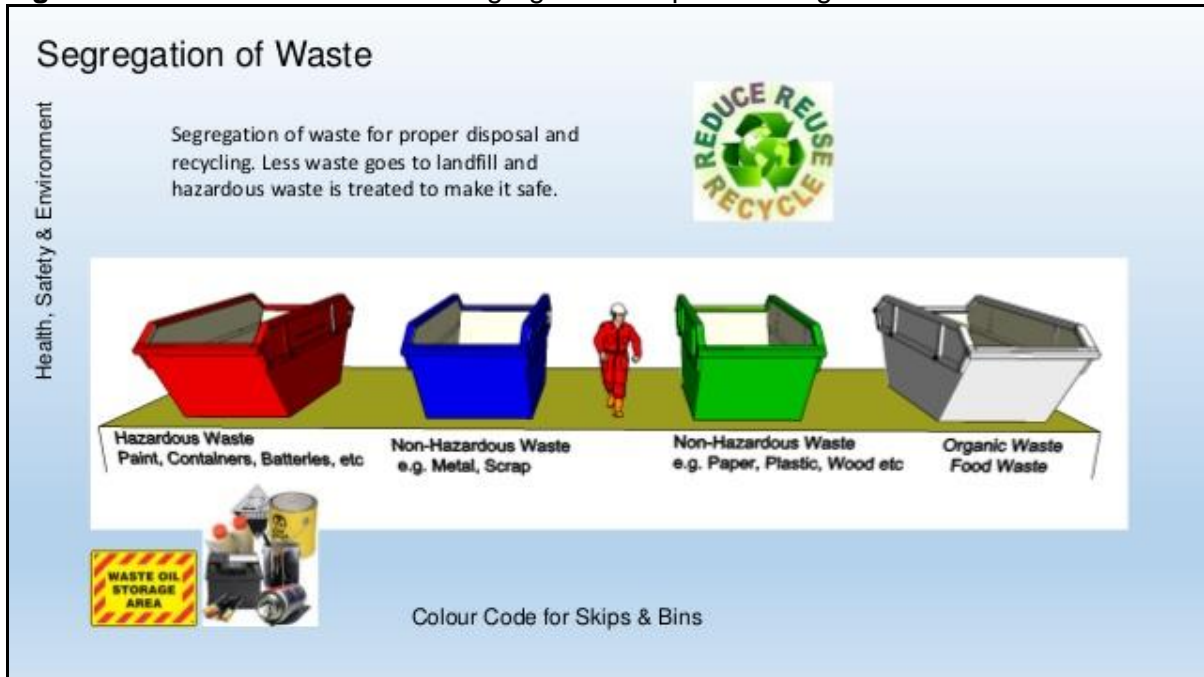
Figure 2 Construction waste segregation compound design
